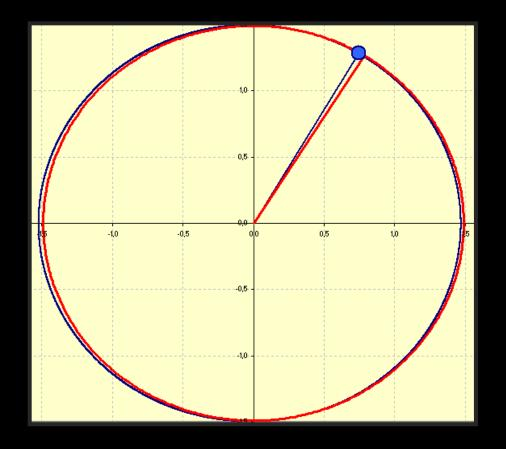
On each day of the year this difference is proportional to the difference between the angle corresponding to the position of the Earth on its trajectory and a reference angle corresponding to the uniform circular movement.
