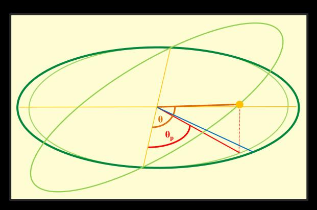
The projection of the apparent annual movement of the Sun on the plane of the celestial equator is no longer a uniform circular movement, that is, the projected angle  $\theta_p$  does not vary in a uniform way over time.
