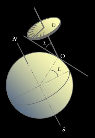
Let us imagine an instrument consisting of a disk D crossed by an axis that is perpendicular to it, placed in a local O of the Earth's surface with latitude L.
