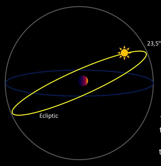
Viewed from Earth, the center of the Sun is projected at a point on the celestial sphere. Throughout the year this projection describes a line, the ecliptic. The plane of the ecliptic makes with the plane of the celestial equator an angle of about 23,5 degrees.
