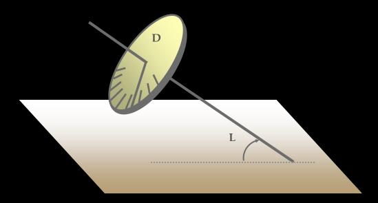
This instrument is an equatorial sundial, since the plane containing the graduated disk is parallel to the equatorial plane. It is possible to build variants of sundials with gnomon parallel to the Earth's axis by changing the position of the dial plane as well as its shape.
