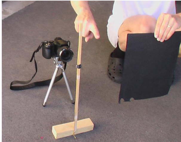
Figure 5. An object is used to shadow the lens, but allows the light from the stars to reach the camera.
